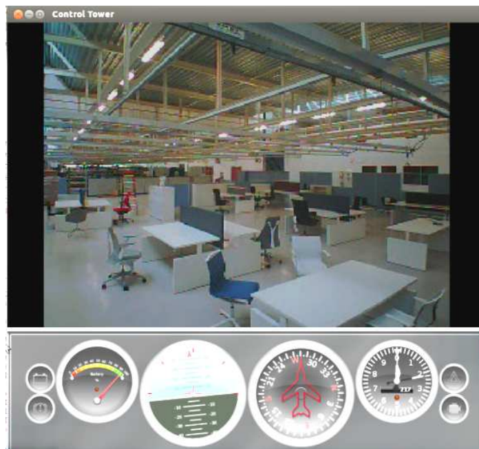
Figure 3: Impression of the AR Drone Control Centre, to which the AR Drone streams the images over the multihop ad hoc network.
