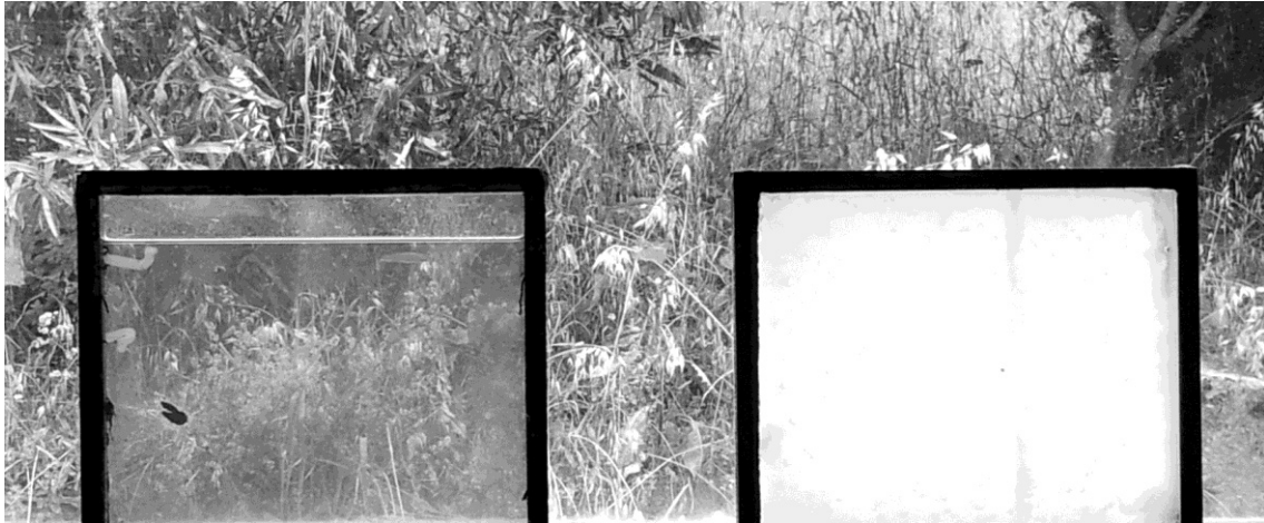
Fig. 1. Samples of DGU_PCM systems used to carry out the optical characterization of PCM glazing systems: on the left, the PCM layer in liquid state; on the right, in solid state.
