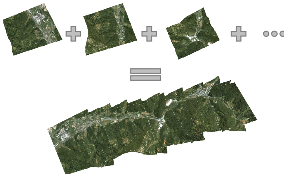
Figure 10. An example of the final mosaic obtained stitching several orthorectified images.
