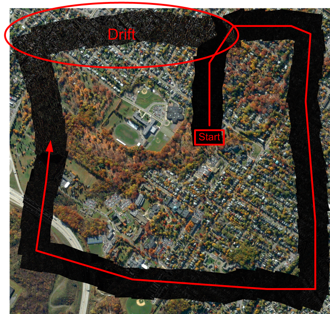
Figure 6. Difference between a reference ortho-photo and a mosaic strip showing the increasing drift in the final part.
