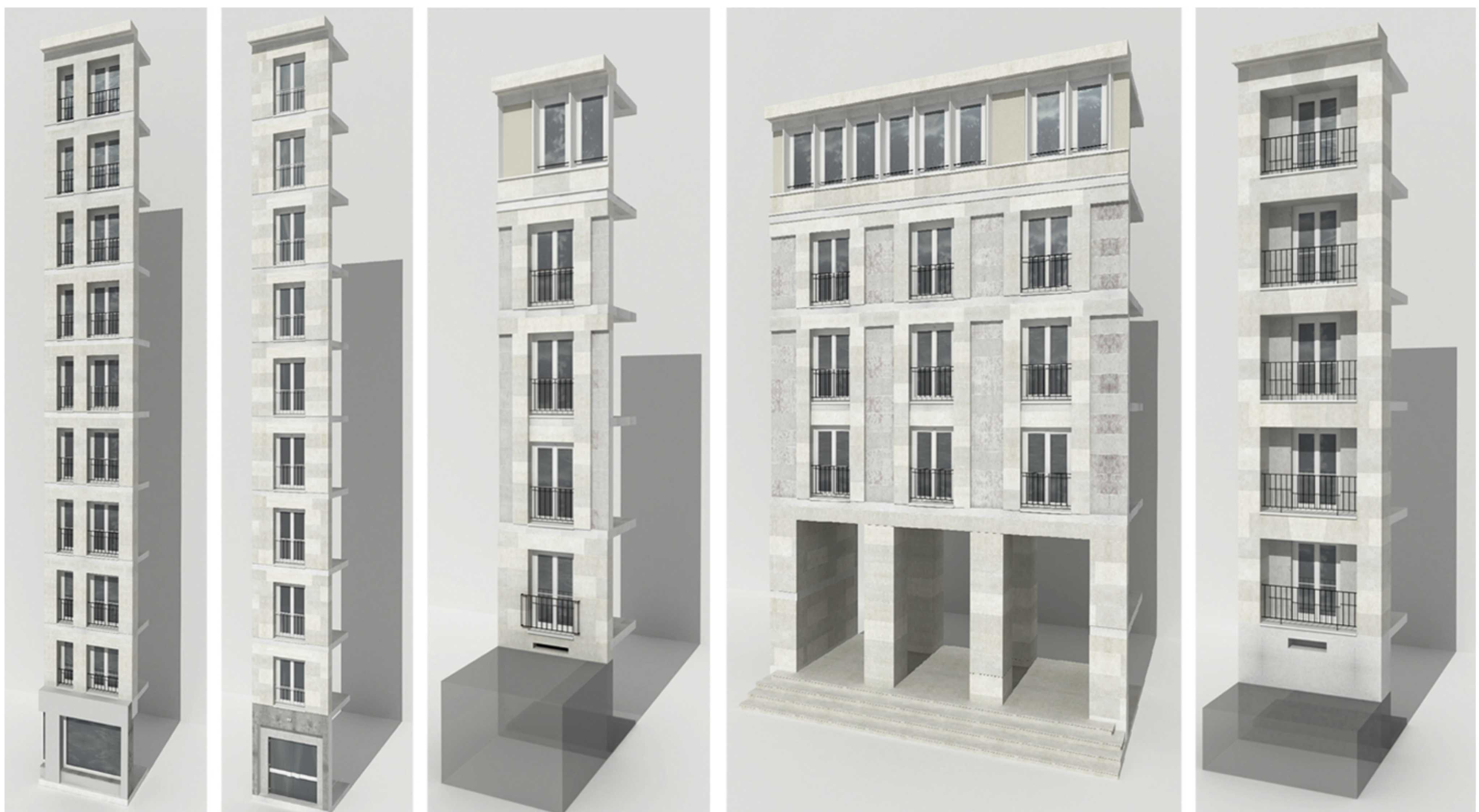
Typological evolution of the stone façade: relationship form - structure
