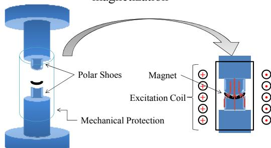
Fig. 3 – Adopted magnetic circuit for the radial magnetization
