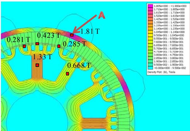
Fig. 7 – Flux density distribution (radial bonded magnet motor)
