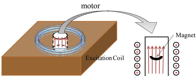
Fig. 2 – Required magnetic circuit for the parallel magnetization
