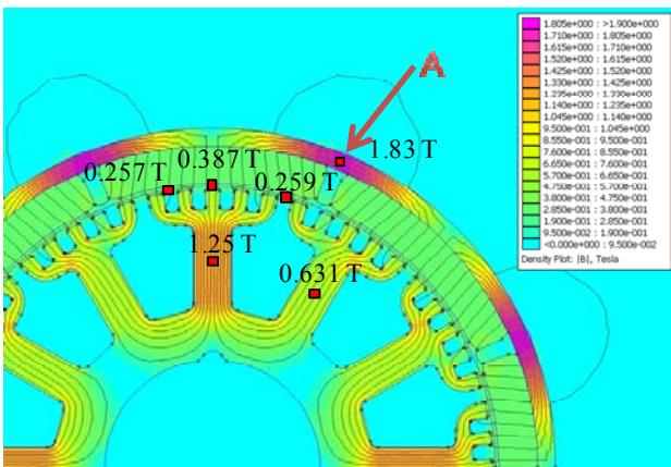
Fig. 6 – Flux density distribution (parallel bonded magnet motor)
