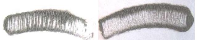
Fig. 5 – Magnetized samples: left parallel, right radial
