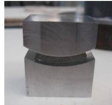
Fig. 4 – Polar shoes around the magnet
