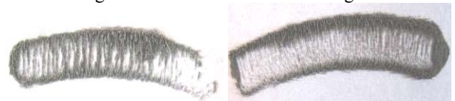
Fig. 5 – Magnetized samples: left parallel, right radial
