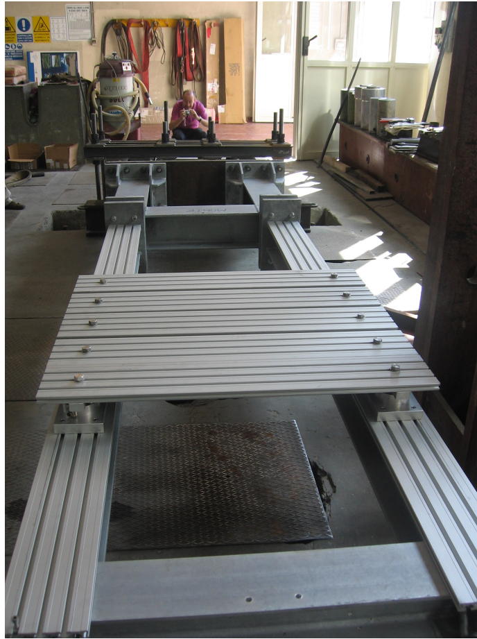
Figure 6: The obstacle mounted in horizontal position as tested in the laboratory.
