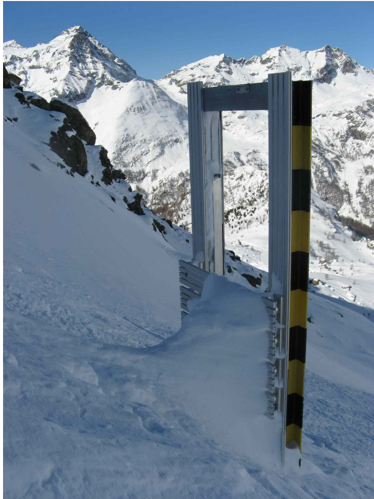
Figure 4: View of the obstacle after an avalanche event. Only the upper part of the steel structure emerges from the snowpack.
