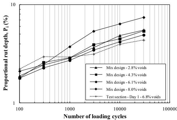
Fig. 3. Wheel-tracking test results
