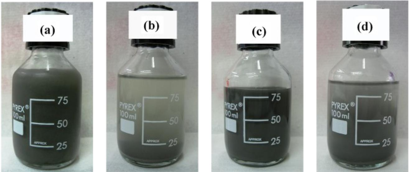
**Fig. 11** Thermal effect on sedimentation of 20 g/L MZVI in BMS (XG/GG = 1:1): (a) and (b) H4 in 1.5 g/L BMS at 20°C after 48 h and at 35°C after 0.5 h, respectively; (c) and (d) B200 in 0.75 g/L BMS at 20°C after 48 h and at 40°C after 0.5 hour, respectively.
