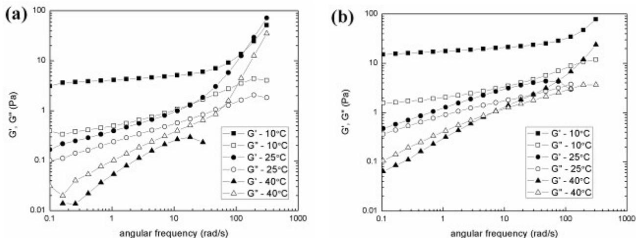
**Fig. 7**  $G'$  and  $G''$  as a function of angular frequency for BMS with a XG/GG weight ratio of 1:1 at a polymer concentration of (a) 1.5 g/L and (b) 3 g/L
