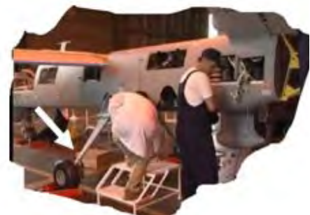
Figure 18. example of tapered leaf spring landing gear
