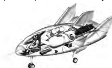
Figure 4b). Martin Marietta X24A internal systems
