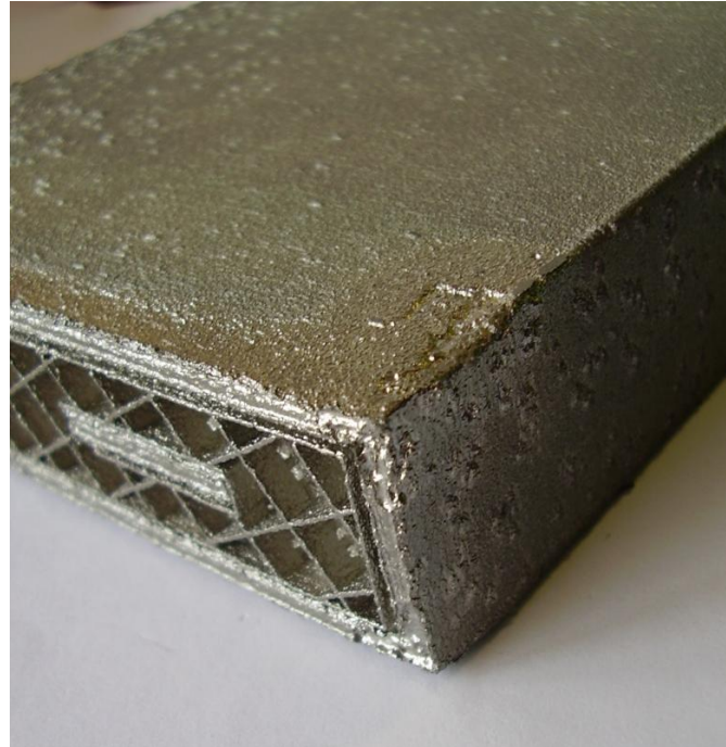
Figure 1: EBM sintered workpiece, as supplied
