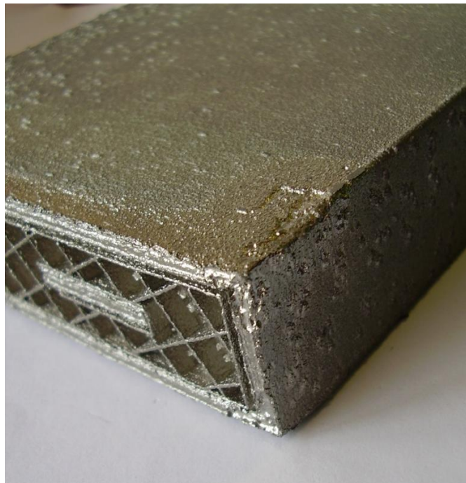
Figure 1: EBM sintered workpiece, as supplied.
