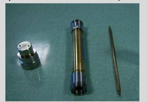
Length 10.5 cm shield conductor radii 3.5 mm Inner conductor radii 1.5 mm
