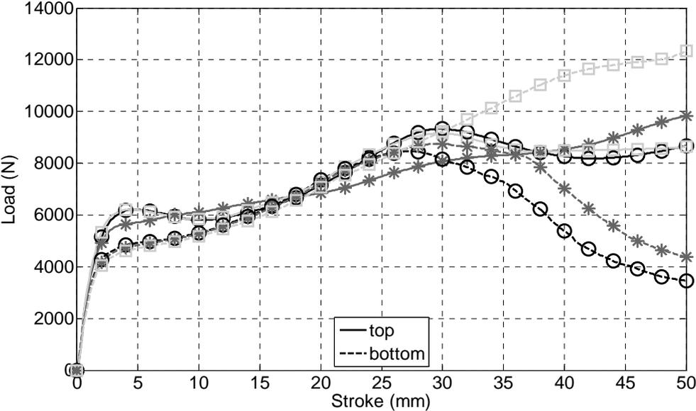
Figure 13: force-displacement curves for the metal specimens joined by spot weld
