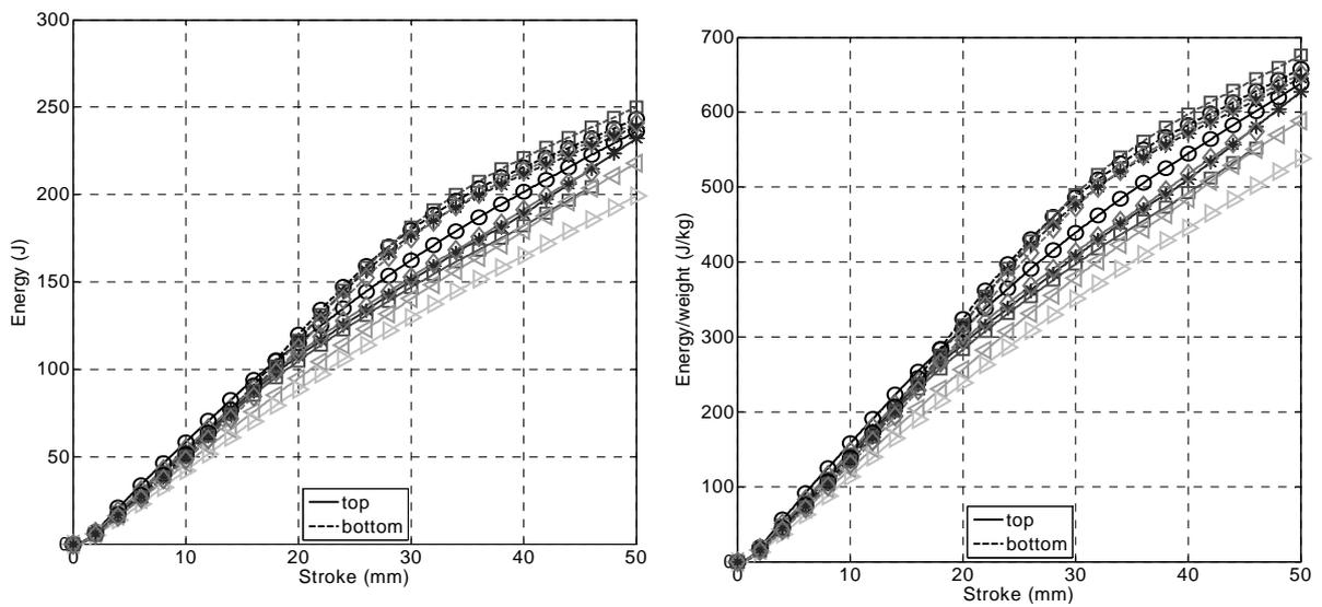
Figure 8: absorbed energy (on the left) and absorbed energy/weight of specimen (on the right) versus displacement for the hybrid specimens
