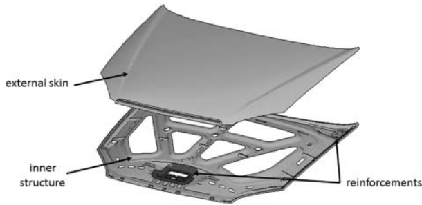
Figure 1. Structure of the reference steel bonnet.
