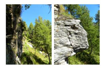
Figure 7.28: Details of the main scarp: vertical cliff where blocks are defined by the main joint sets.
