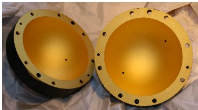
Figure 2.2: Image of the interior cavity surface of the resonator.
