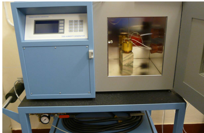
Figure 4.6: The commercial two-pressure humidity generator (Thunder Scientific Corporation mod 2500) used in the experiment with the microwave resonator in the test chamber.
