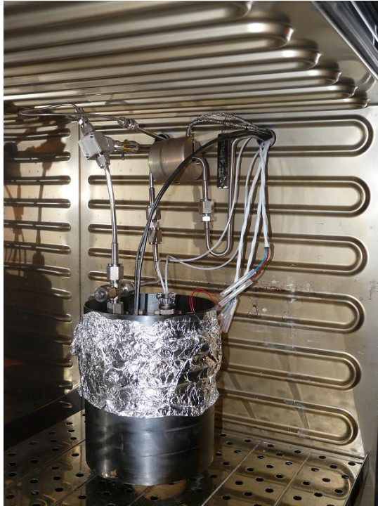
Figure 3.6: Image of the experimental set up inside the oven. The stainless steel vessel and the differential pressure transducer can be observed.
