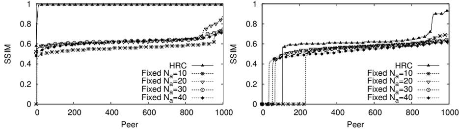
Figure 11: Average SSIM per peer distribution for HRC and non-adaptive schemes for video rates  $r_s = 800\text{kb/s}$  (left) and  $r_s = 1600\text{kb/s}$  (right). Experimental results in swarm of 1000 peers.
