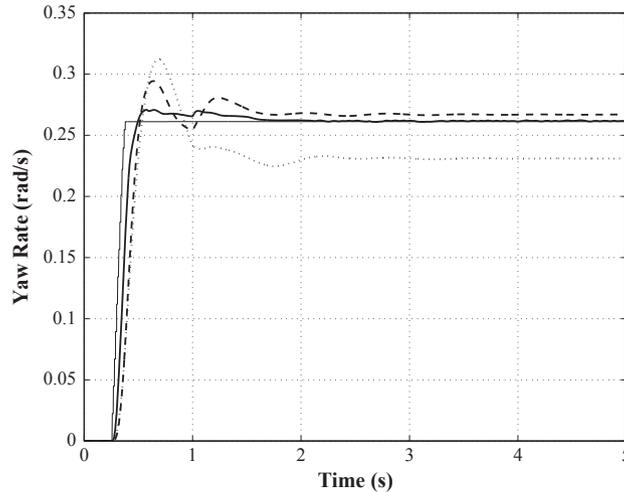
Figure 4. Results of the  $50^\circ$  handwheel step test when a blust of wind occurs at 1 s. Uncontrolled vehicle yaw rate (dotted), reference yaw rate (thin solid line), and yaw rate obtained with the Set Membership Predictive Control (solid) and Nonlinear Model Predictive Control based on a physical model (dashed) control laws.
