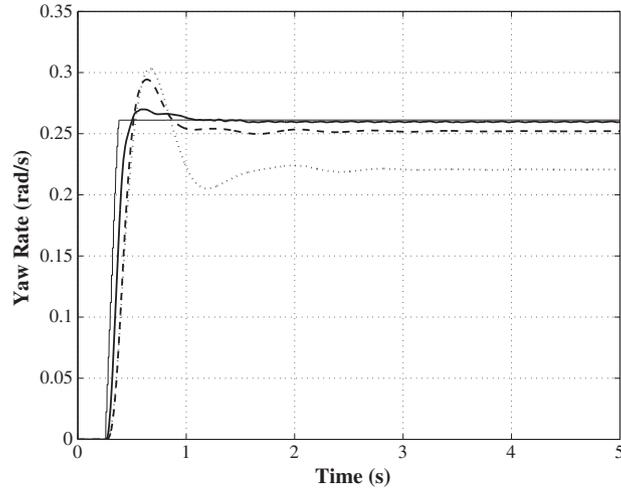
Figure 2. Results of the  $50^\circ$  handwheel step test with nominal parameters. Uncontrolled vehicle yaw rate (dotted), reference yaw rate (thin solid line), and yaw rate are obtained with the Set Membership Predictive Control (solid) and Nonlinear Model Predictive Control based on a physical model (dashed) control laws.
