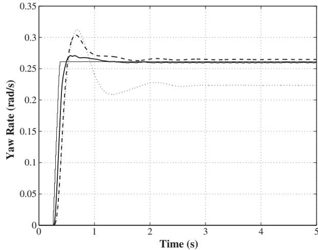
Figure 3. Results of the  $50^\circ$  handwheel step test with increased mass. Uncontrolled vehicle yaw rate (dotted), reference yaw rate (thin solid line), and yaw rate are obtained with the Set Membership Predictive Control (solid) and Nonlinear Model Predictive Control based on a physical model (dashed) control laws.
