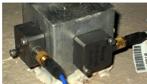
Figure 4.32 - Metallic cube used to locate the accelerometers in triaxial position.
