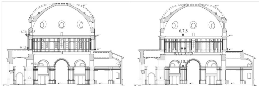
Figure 4.18 - Arrangement of sensors in the various setups: (a) setup 1, (b) setups from 2 to 4, (c) setups 5 and 6. Fixed nodes for linking shapes were in 0,1,2 (a triaxial geophone).
