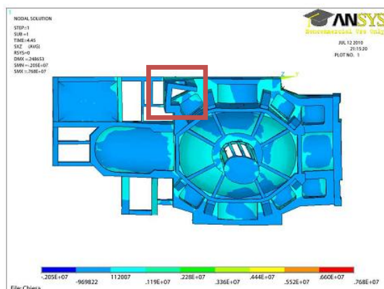
Figure 4.42 - Time history analysis, notice the deformation of the bell tower (emphasised in red).
