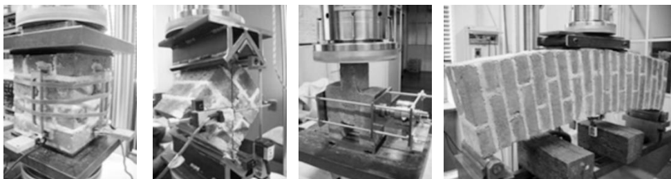
Figure 7.3 - Tests conducted on the masonry samples.
