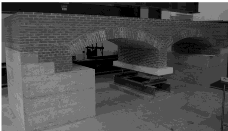
Figure 7.1 - The scaled masonry bridge: notice the settlement application device under the central pier.
