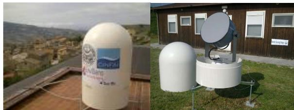
**Figure 1.** The X-band mini radar with and without the radome.
