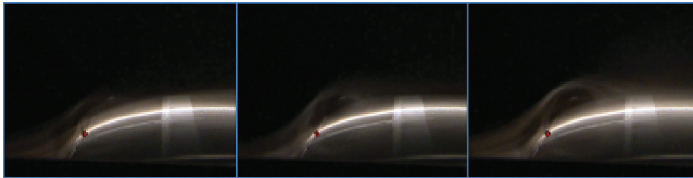
Figure 19. Bubble size unsteadiness. \alpha = 3^\circ , Re = 265000 , (x/c)_{\text{slit}} = 1.25\% , F^+ = 3.2 .
