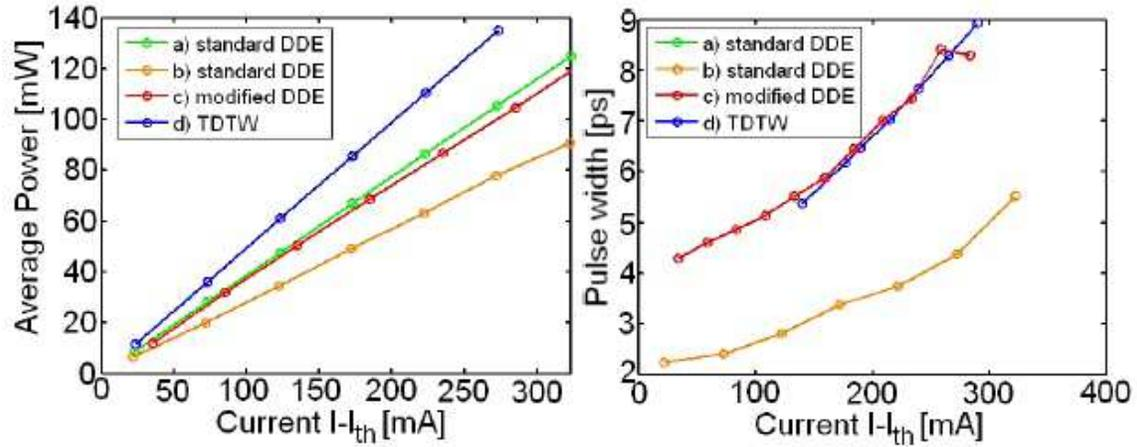
**Fig.2** Average power and pulse width vs. current obtained at a fixed 7V SA voltage for the structures reported in Fig.1, using respectively a standard DDE model (a-b), the proposed multi-section DDE model (c) and the FDTW model (d). Structure (a) (green) shows a continuous-wave operating regime.
