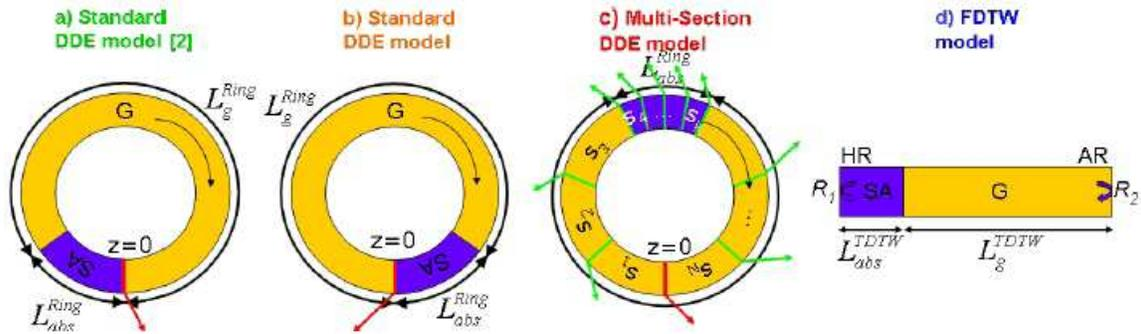
**Fig.1** (a-b) Scheme of ring lasers described by a standard DDE model; (c) ring laser simulated by the multi-section DDE model; (d) schematics of FP laser modelled via the FDTW model.
