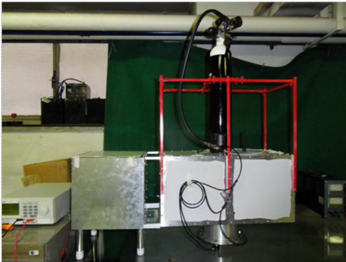
Figure 23. Test of separation between the Occulting and Observing engineering models.
