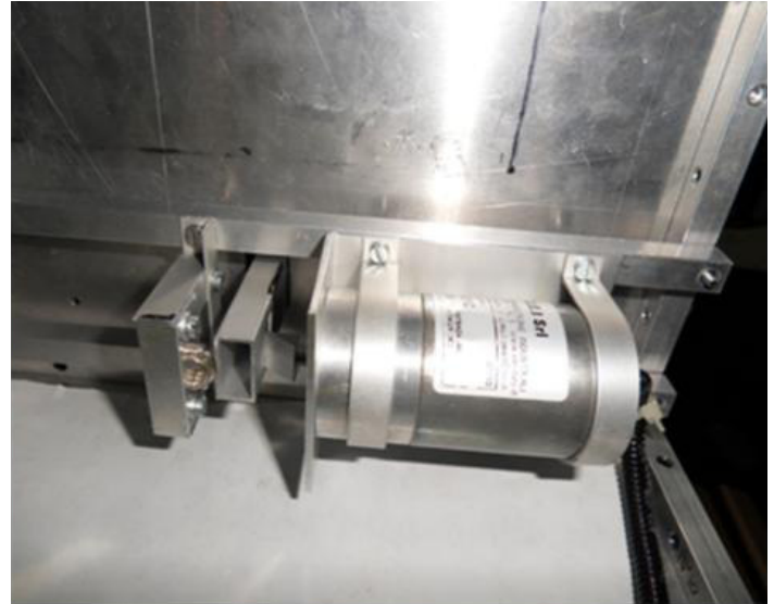
Figure 24. Undocking/separation subsystem: the latch.
