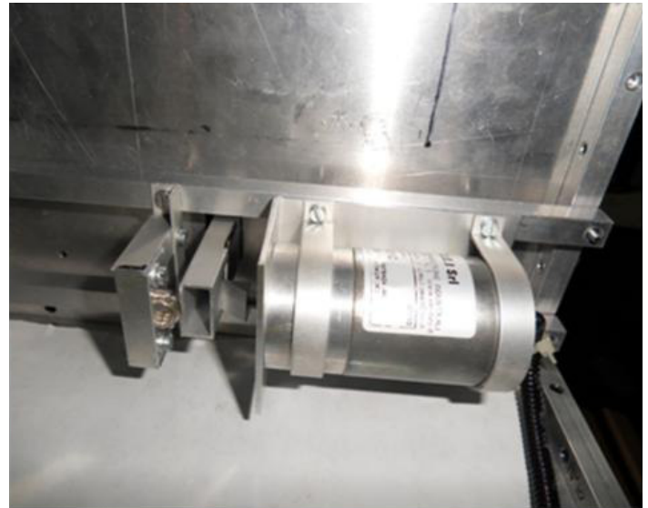
Figure 24. Undocking/separation subsystem: the latch.
