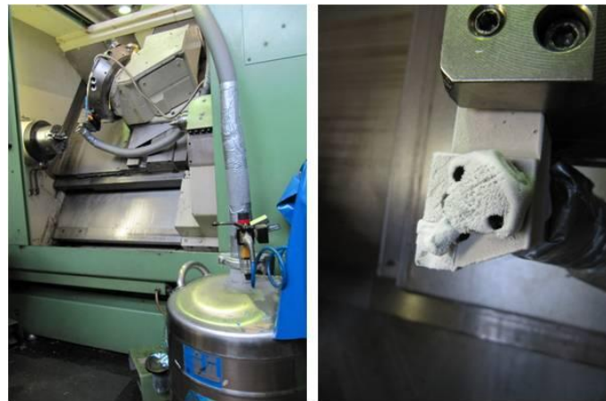
Figure 3: Experimental set-up with cryogenic lubrication equipment. The detail shows a CNMA insert at the end of a cutting test
