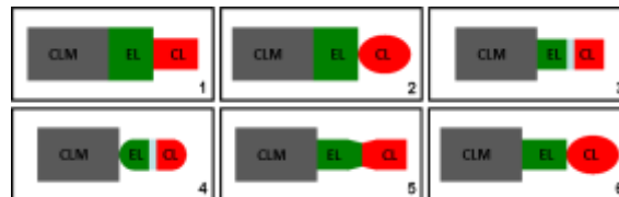
Fig. 5: Alternative airlock configurations: 1) EL integrated with HAB plus rigid CL; 2) EL integrated with HAB plus inflatable CL; 3) unique rigid module for both EL and CL separate internally through a bulkhead; 4) unique inflatable module for both EL and CL separate internally through a bulkhead; 5) independent rigid EL and rigid CL; 6) independent rigid EL and inflatable CL.
