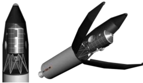
Fig. 3: HAB interfaces with the Hyperion launcher
