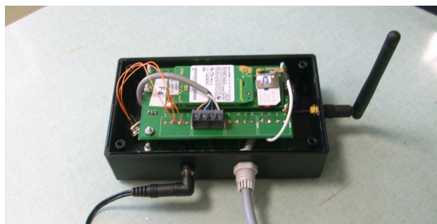
Figure 3. The GPRS based data acquisition system.
