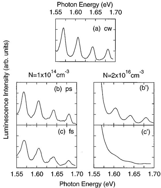
FIG. 2. Spectra of band-to-acceptor luminescence from *p*-type GaAs at a temperature of  $T_L = 10$  K for different excitation conditions. The spectra were measured with (a) continuous wave, (b) 20 ps, and (c) 150-fs excitation of  $N_{\text{ex}} = 10^{14}$  electrons per  $\text{cm}^3$  (photon energy 1.73 eV). Parts (b') and (c') give results for  $N_{\text{ex}} = 2 \times 10^{16}$   $\text{cm}^{-3}$ .
