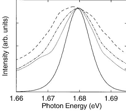
FIG. 4. Spectral profile of the first luminescence peak for carrier densities of  $N=8 \times 10^{13} \text{ cm}^{-3}$  (dotted line),  $5 \times 10^{14} \text{ cm}^{-3}$  (dash-dotted line), and  $4 \times 10^{15} \text{ cm}^{-3}$  (dashed line). For comparison, the spectral envelope of the femtosecond excitation pulses is shown (shifted to lower photon energy by 50 meV, solid line).
