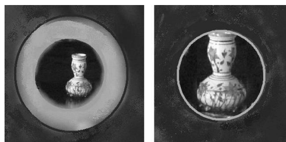
Figure 4: A “room version” of the sketch in Figure 3 , obtained with the pair (3',5) of a dodecahedron made of cardboard. The vase is 0.2 m high and, when we see the coincidence as the image on the right, according to Table 1 the dodecahedron is at a distance of 2.5 m from it.
