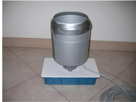
FIGURA 75: PLUVIOGRAFO INTERRATO
