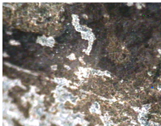
Figure 18. Hot salt corrosion on an AISI 321 specimen after 20 ageing cycles (800x magnification).
