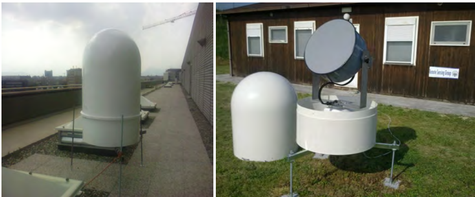
Fig. 1. The portable, low-cost weather radar with (left picture) and without (right picture) the 1-meter Diameter radome. The configuration shown here is the so-called “super-gauge”, which is a single-elevation scanning in the horizontal plane with a 3.6° beam width paraboloid (Diameter of the paraboloid is 0.6 m).
