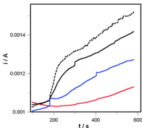
**Fig. 2** Current vs. time curve for the FTO/Nafion/CoAPO5 photoanode under different illumination conditions (Scheme S2 (ESI†) for setup): (i) dark room conditions (red curve); (ii) transversal illumination (blue curve); (iii) direct illumination (black curve); (iv) reverse illumination (broken curve). Solution: 0.1 M  $\text{K}_2\text{SO}_4$  in water. Light program: 0–180 s dark; 180–580 s with light intensity of  $1000 \text{ W m}^{-2}$ .  $E = +1.6 \text{ V vs. Ag/AgCl}$ .
