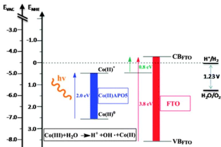
**Scheme 1** Basic diagram of the states involved in photoinduced electron transfer from the fundamental level of CoAPO5 to the conduction band of FTO. Note that under illumination a minimum bias of 0.8 V is necessary to obtain a photocurrent.
