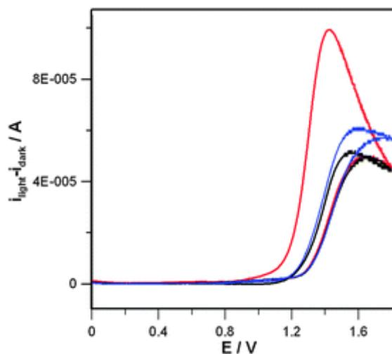
**Fig. 3** Photocurrent vs.  $E$  curve for the FTO/Nafion®/CoAPO5 photoanode during three successive voltammetric scans. Red curve: first cycle; blue curve: second cycle; black curve: third cycle. Experimental conditions are the same as already described in [Fig. 1 and 2](#). The photocurrent has been calculated by subtracting the stationary CV in the dark from the one recorded under frontal illumination.
