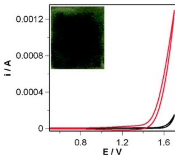
**Fig. 1** Cyclic voltammetric curves of FTO slides ( $R = 30 \text{ Ohm} \times \text{cm}$ ) coated by Nafion® films only (blank, black curves) and Nafion/CoAPO5 films (red curves). Solution: 0.1 M  $\text{K}_2\text{SO}_4$  in water. Scan rate  $0.1 \text{ V s}^{-1}$ . 20 mg of catalyst was added on the slide dispersed in 0.3 mL of 5% w/w Nafion® isopropanol solution. Inset: picture of the FTO/Nafion/CoAPO5 photoanode.
