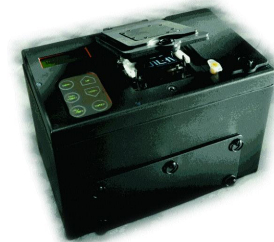
Figure 1.1 Fiber-optic, fully automated biosensor performs four immunoassays simultaneously in 5 to 10 minutes and shows the results on an LCD screen in words
