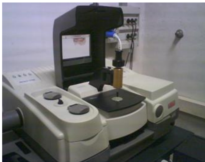
Figure 6.6 Attenuated Total Reflection-Fourier Transform Infra Red spectroscopy
