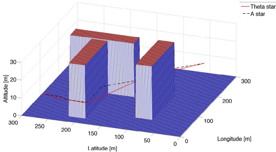
Figure 2.18. Comparison between Theta\* and A\* (3D view)
