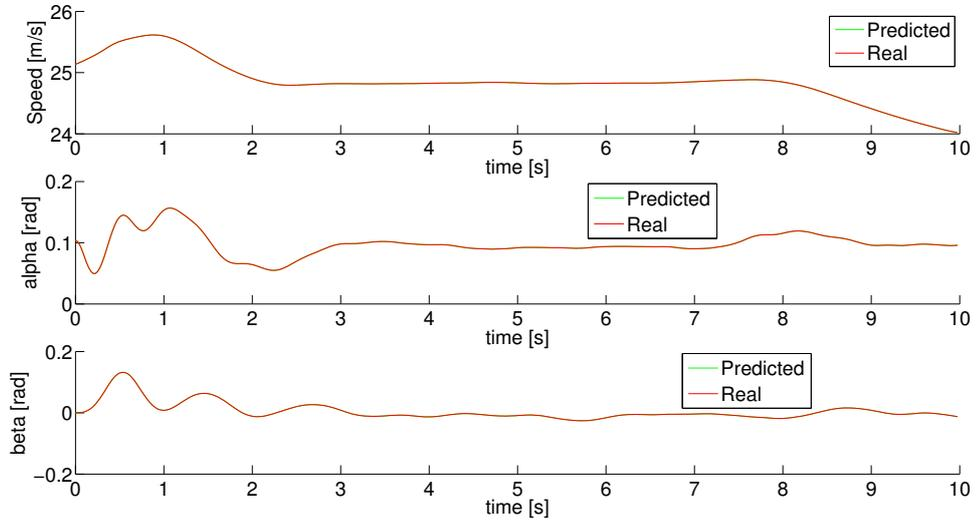
Figure 6.28. Comparison between predicted and real relative-wind speed, angle of bank and attack
