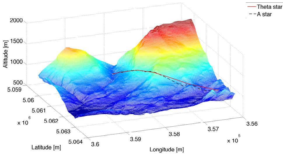
Figure 2.15. Comparison between Theta\* and A\* (3D view)
