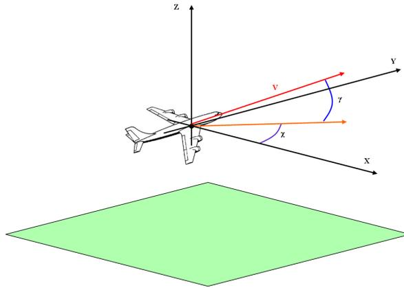
Figure 4.1. The Ground Reference frame (G frame)
