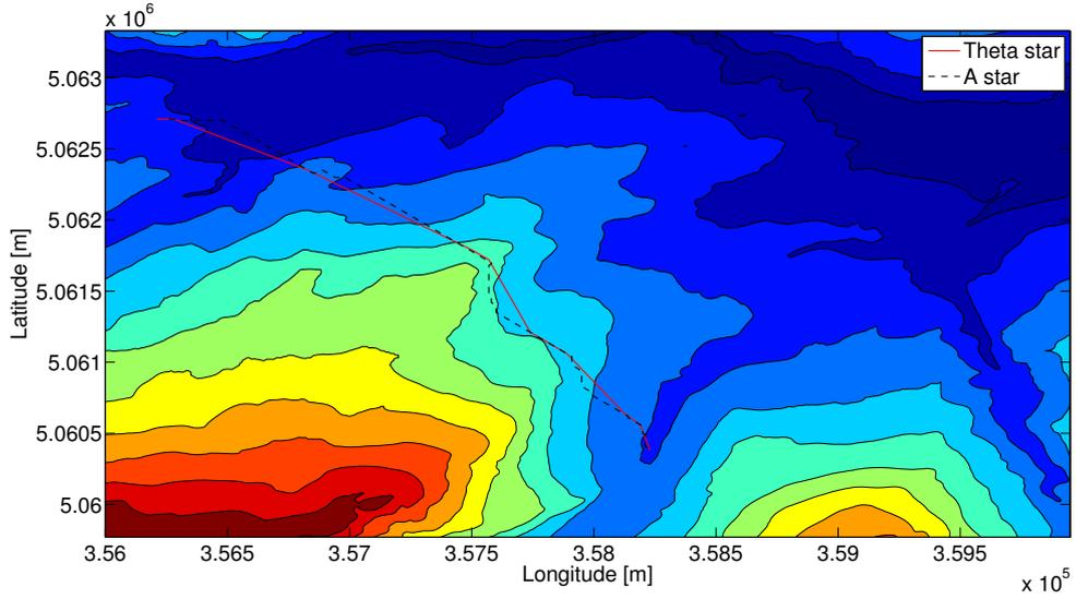
Figure 2.16. Comparison between Theta\* and A\* (Longitude-Latitude plane)
