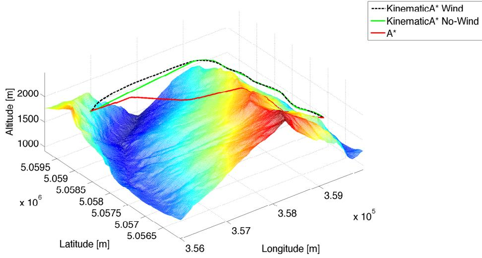
Figure 5.3. An example of paths generated with  $KA^*$  on a highland environment compared with the one generated with  $A^*$ .
