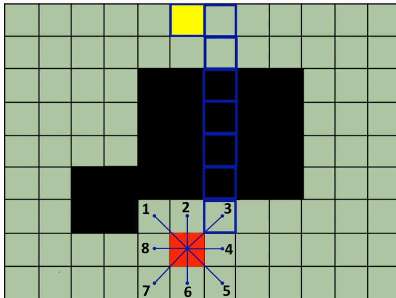
Figure 2.5. Eight connections of the starting node.
