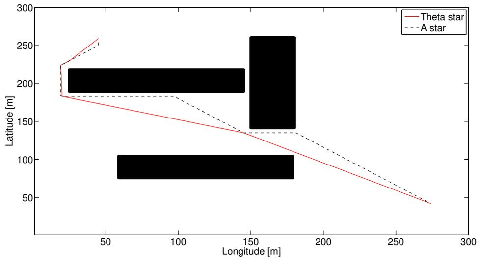
Figure 2.19. Comparison between Theta\* and A\* (Longitude-Latitude plane)
