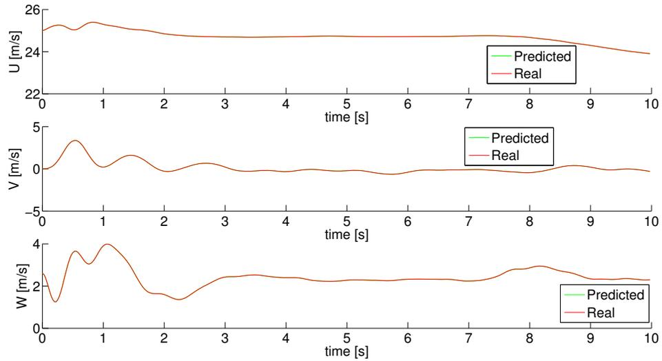
Figure 6.25. Comparison between predicted and real speed
