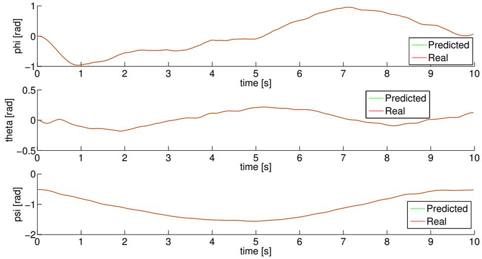
Figure 6.39. Comparison between predicted and real attitude
