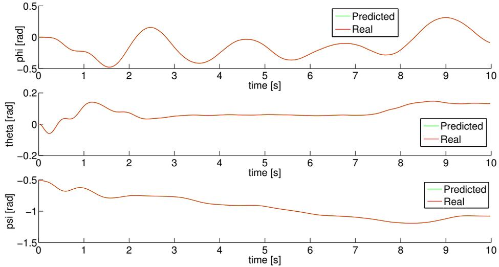
Figure 6.27. Comparison between predicted and real attitude
