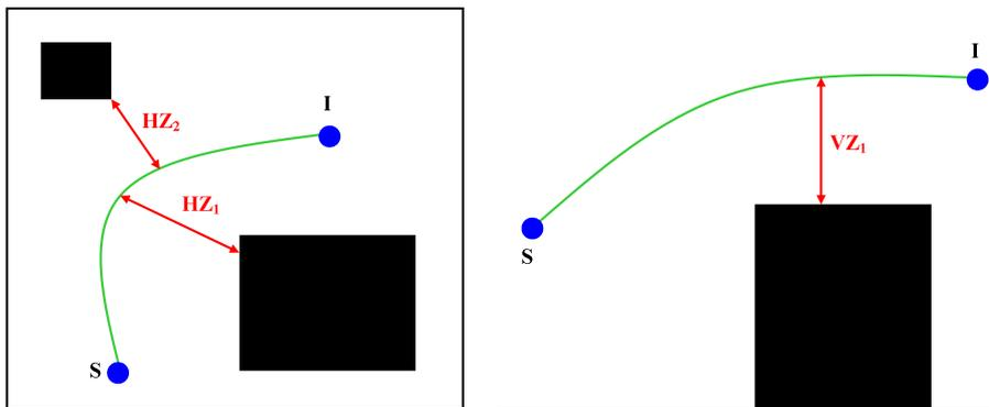
Figure 4.5. Horizontal and Vertical separation from an obstacle
