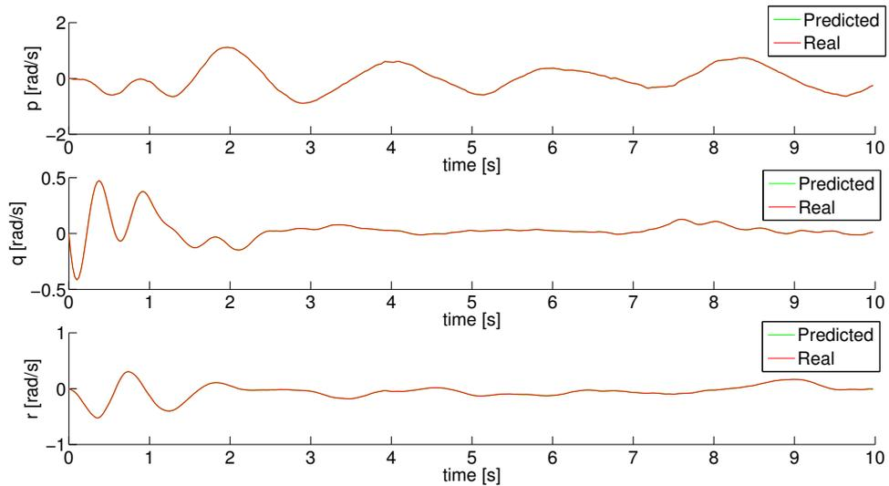
Figure 6.26. Comparison between predicted and real angular rate
