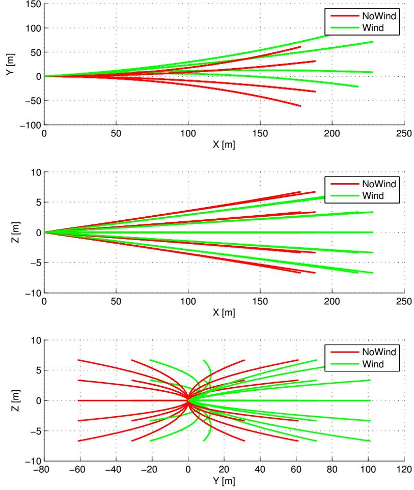
Figure 4.3. Comparison of states evolution (2D view) with and without wind ( $W_x = 5$  [m/s],  $W_y = 5$  [m/s],  $W_z = 0$  [m/s]).
