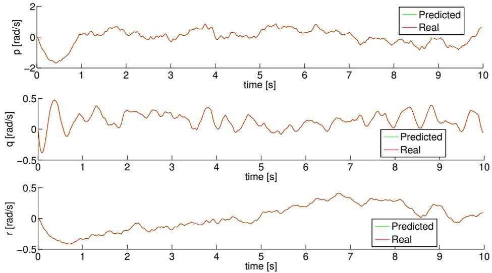
Figure 6.38. Comparison between predicted and real angular rate
