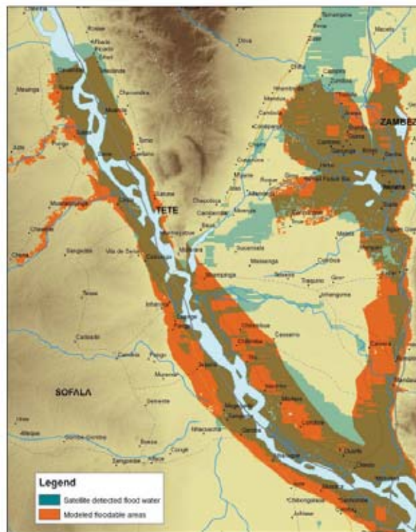
Figure 4.8 – Definition of floodable areas: output example (evaluation of flood extent in Zambezi floodplain for the extreme meteorological event occurred in Mozambique, February 2007).
