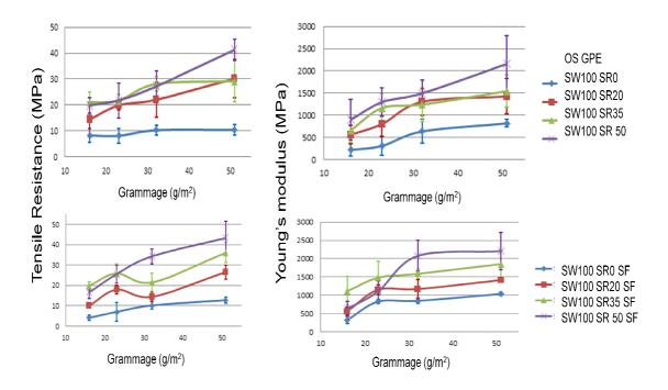
• Tensile resistance (left) and Young's modulus (right) of the One Shot GPE membranes reinforced with the handsheets of the refining series prepared with HW fibers (HW100) with (top) and without (bottom) short elements as a function of the grammage
