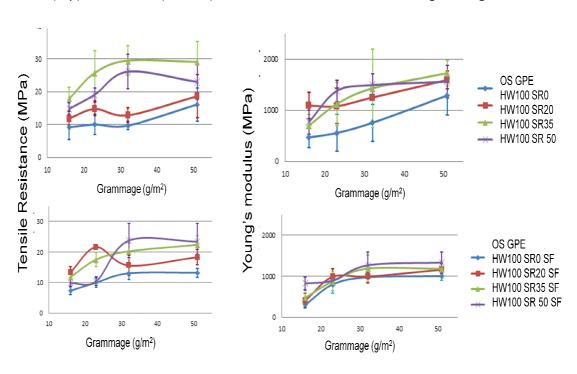
Tensile resistance (left) and Young's modulus (right) of the One Shot GPE membranes reinforced with the handsheets of the refining series prepared with the mixture of fibers HW:SW (60:40) (SW40) with (top) and without (bottom) short elements as a function of the grammage
