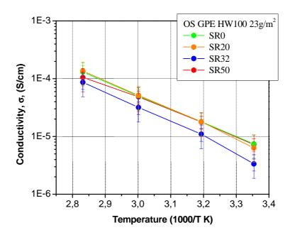
Arrhenius plots of the conductivity of One shot GPEs reinforced with handsheets with grammage 23gm<sup>-2</sup> containing fibres HW (HW100), with different refining degrees without short elements.
