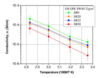
• Arrhenius plots of the conductivity of One shot GPEs reinforced with handsheets with grammage 23gm<sup>-2</sup> containing the mixture of fibres HW:SW (60:40), with different refining degrees without short elements.
