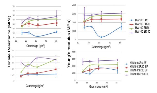
• Tensile resistance (left) and Young's modulus (right) of the hansheet refining series prepared with the mixture of fibers HW:SW (60:40) (SW40) with (top) and without (bottom) short elements as a function of the grammage
