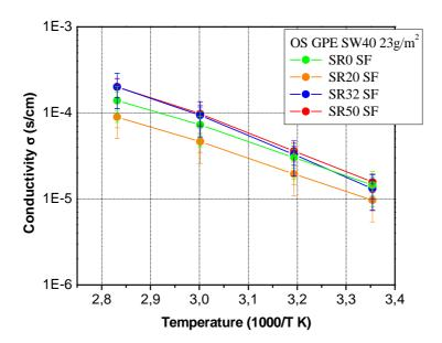
• Arrhenius plots of the conductivity of One shot GPEs reinforced with handsheets with grammage 23gm<sup>-2</sup> containing fibres HW (HW100), with different refining degrees.
