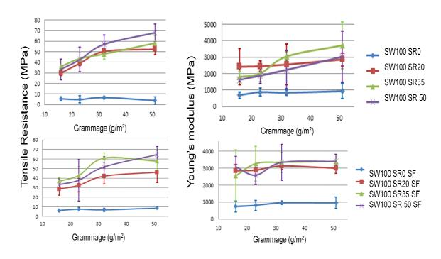
• Tensile resistance (left) and Young's modulus (right) of the hansheet refining series prepared with HW fibers (HW100) with (top) and without (bottom) short elements as a function of the grammage
