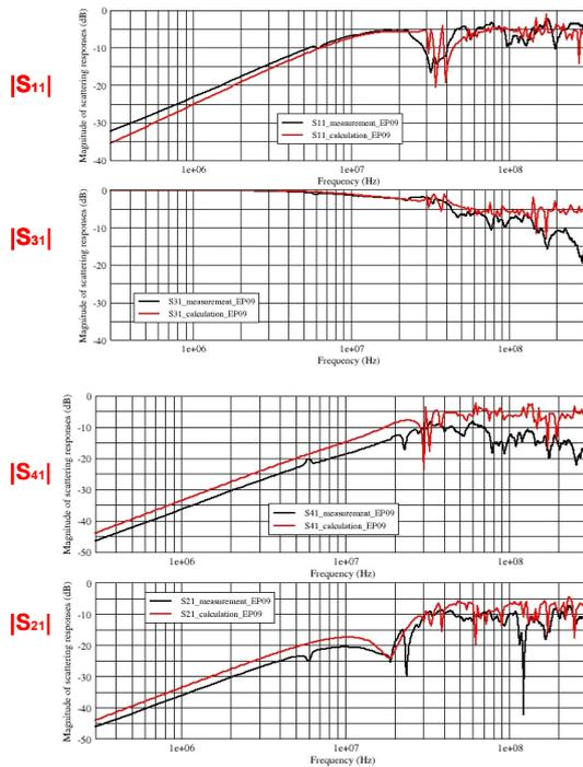
Figure 9: Scattering response of a single wire and a shielded twisted pair cable (configuration S7TW5 of Fig.4) considering in input signal at port 1". From top to bottom:  $S_{11}$ ,  $S_{31}$ ,  $S_{41}$  and  $S_{21}$
