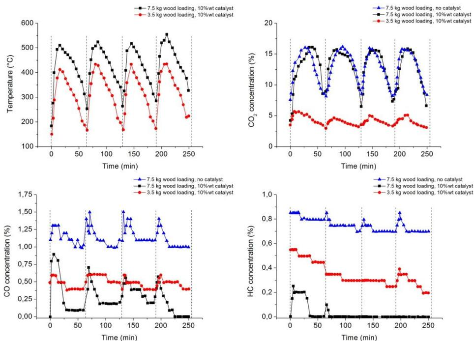
**Figure 6.** Top: stove operating temperature and CO<sub>2</sub> emissions; bottom: CO and HC oxidation tests with and without the full-scale catalyzed monolith.
