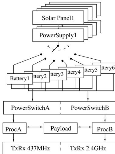
Fig. 2. PiCPoT internal structure
