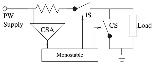
Fig. 5. Block diagram of latchup protection circuit.
