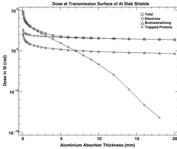
Fig. 3. Total dose radiation diagram with respect to the shield thickness in LEO orbit.
