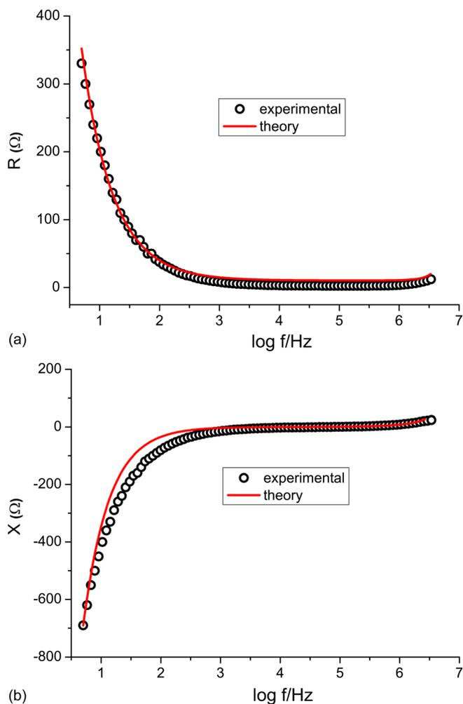
FIG. 5. (Color online) Real,  $R$ , and imaginary,  $X$ , parts of the electrical impedance of the hydrogel 4% HEC, 3% NaCl. The data refer to a sample with  $d=0.57$  mm and  $S=5 \times 10^{-5}$  m<sup>2</sup>. The best fit parameters are  $D_0=0.25 \times 10^{-10}$  m<sup>2</sup>/s,  $N_0=3.4 \times 10^{26}$  m<sup>-3</sup>,  $s=9 \times 10^{10}$  1/(m V s).
