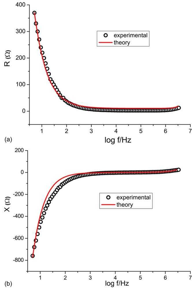
FIG. 4. (Color online) Real,  $R$ , and imaginary,  $X$ , parts of the electrical impedance of the hydrogel 2% HEC, 3% NaCl. The data refer to a sample with  $d = 0.54$  mm and  $S = 5 \times 10^{-5}$  m<sup>2</sup>. The best fit parameters are  $D_0 = 0.22 \times 10^{-10}$  m<sup>2</sup>/s,  $N_0 = 3.6 \times 10^{26}$  m<sup>-3</sup>,  $s = 9 \times 10^{10}$  1/(m V s).
