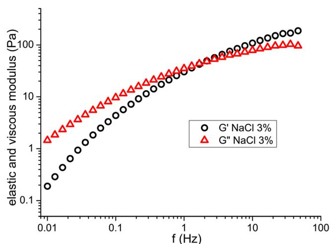
FIG. 2. (Color online)  $G'$  and  $G''$  vs  $f$  for the hydrogel with 2% of HEC and 3% of NaCl. Imposed shear stress  $\sigma = 5$  Pa. Similar results are obtained when the concentration of NaCl is changed. The cut frequency  $f_c \sim 5$  Hz.
