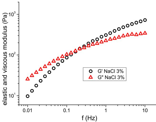
FIG. 3. (Color online)  $G'$  and  $G''$  vs  $f$  for the hydrogel with 4% of HEC and 3% of NaCl. Imposed shear stress  $\sigma = 50$  Pa. Similar results are obtained when the concentration of NaCl is changed. The cut frequency  $f_c \sim 0.5$  Hz.
