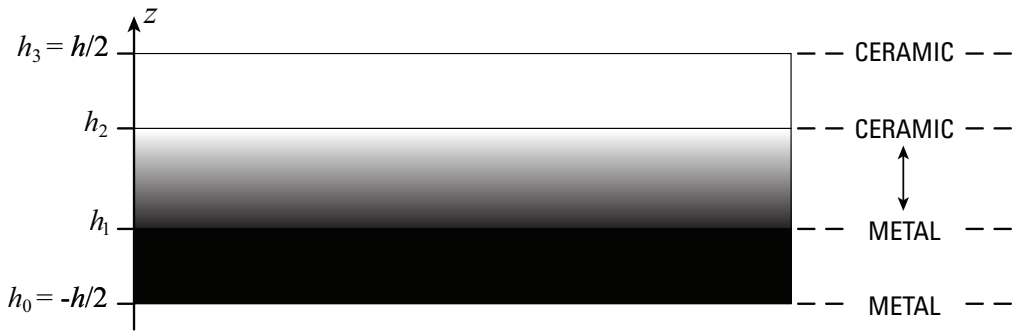
Fig. 3. Plate B: sandwich plate with FGM core and isotropic skins.
