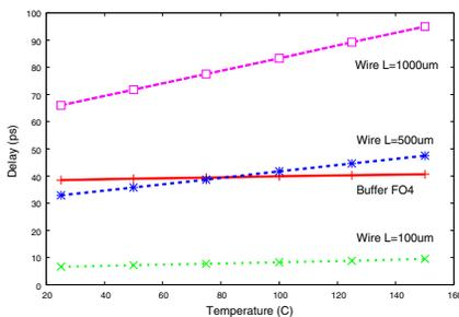
Fig. 5. Temperature induced delay increase in interconnects.
