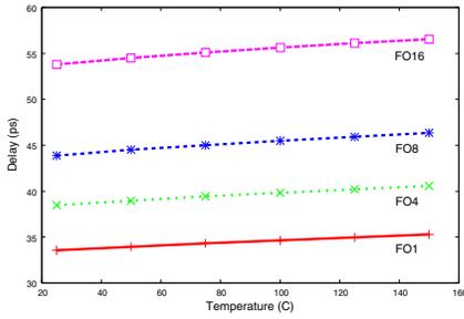
Fig. 4. Temperature induced delay increase in clock buffers.
