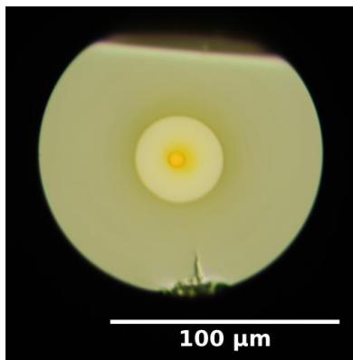
Fig. 2. Optical micrograph of a section of the fabricated tellurite fiber. The triple glass structure, featuring the  $\text{Er}^{3+}/\text{Ce}^{3+}$  doped glass composition TZ3 in the center, is clearly evident.
