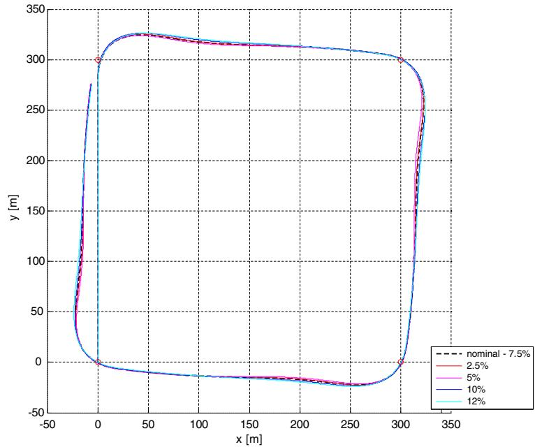
**Fig. 21** The trend of the cross track error with different static margins (square pattern)
