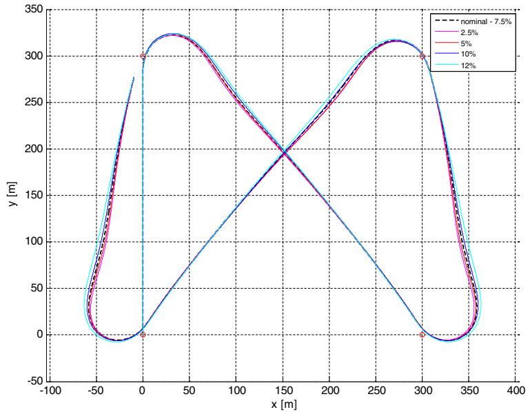
**Fig. 23** The trend of the cross track error with different static margins (butterfly pattern)
