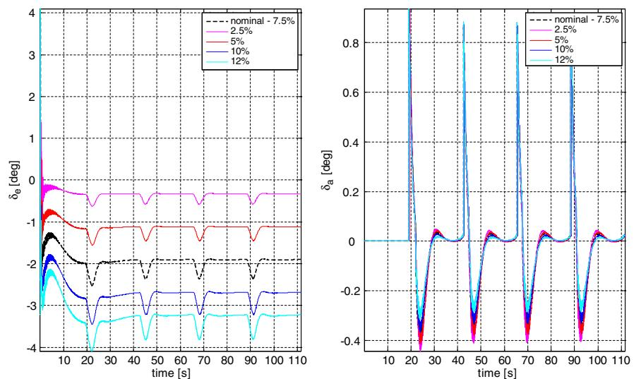
**Fig. 25** Elevon deflection with different static margins (butterfly pattern)
