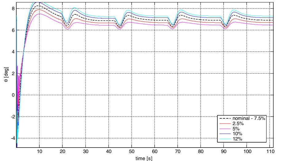
**Fig. 14** The trend of the angle of roll with different static margins (square pattern)
