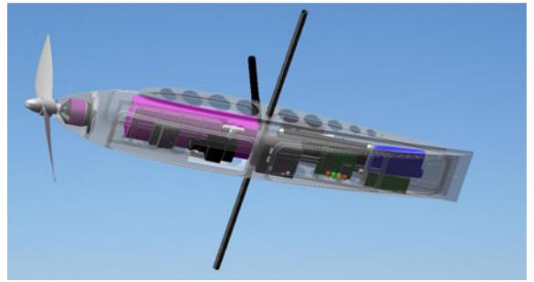
**Fig. 2** The layout of the on-board components
