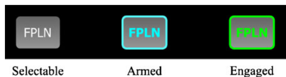
Fig. 8 Autopilot mode pushbutton states
