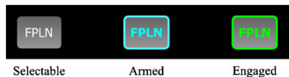
Fig. 8 Autopilot mode pushbutton states
