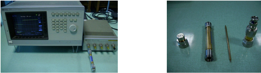
Fig. 15. The frontal panel of the HP 54120B digitalizing oscilloscope with rise time t_r = 10 ps (left). The coaxial probe (Maury Microwave Airline, model no. 2653S10, length \ell = 10.5 cm used in the measurement setup (right).
